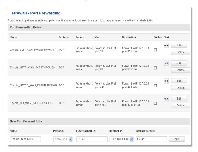
You can use port forwarding to set up servers and services on local LAN machines. The above picture shows how you can set up a rule that would allow a website that is being hosted on 192.168.1.109, to be reached from the outside by entering http://routersExternallp:12345/.
