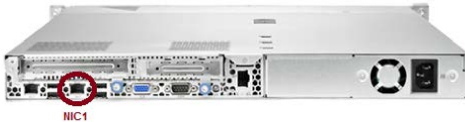
Figure 2-5: First On-board Network Port on HP DL320e Gen 8 Server
