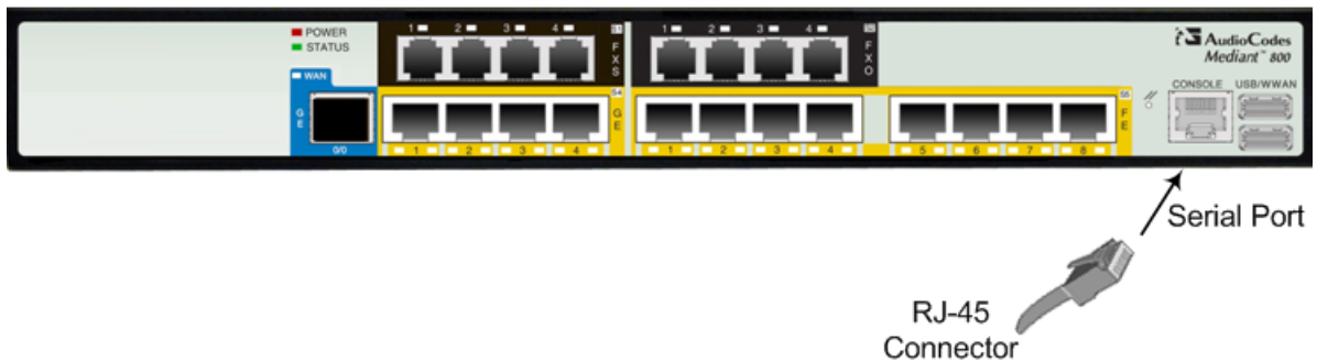
Figure 5-19: Cabling Serial Interface (RJ-45) on Mediant 800B
