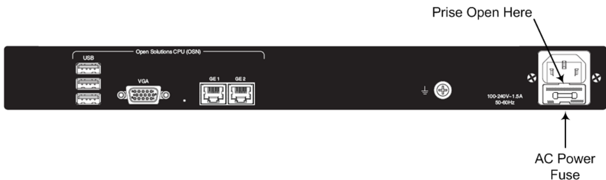
Figure 6-1: Opening the Fuse Cavity
