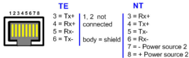
Figure 5-12: RJ-45 Connector Pinouts for BRI Ports
