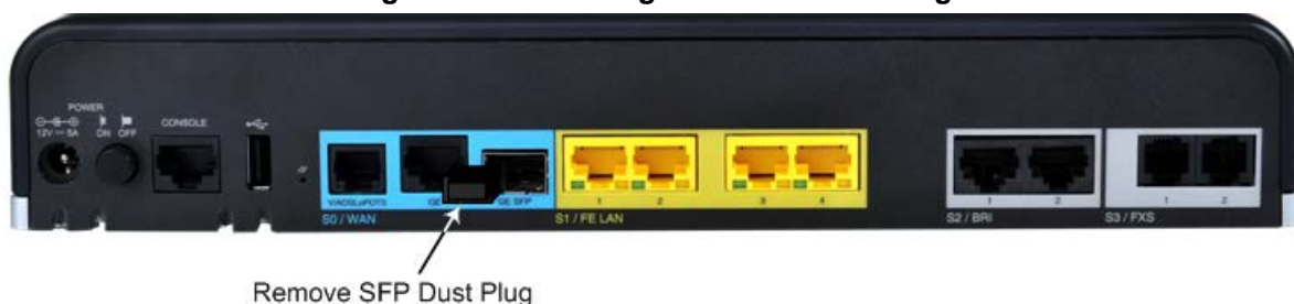
Figure 5-2: Removing Protective Dust Plug
