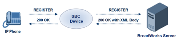
Figure 28-10: Interoperability with BroadWorks Registration Process
