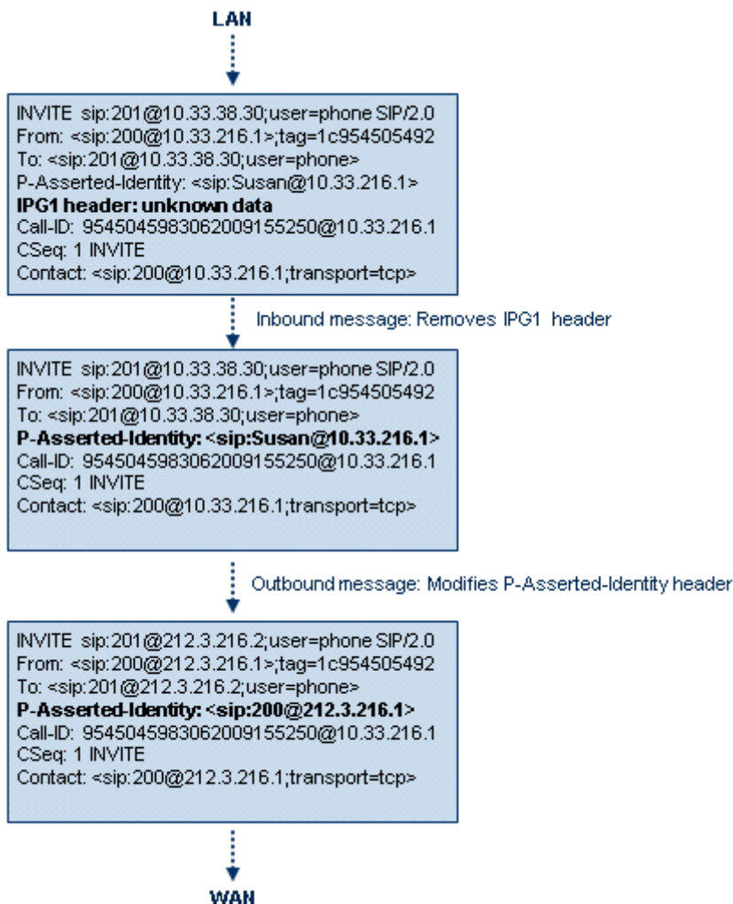
Figure 18-2: SIP Header Manipulation Example
