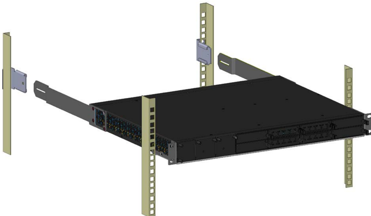
Figure 4-7: Sliding the Rear-Mounting Flanges into the Rear-Mounting Brackets (80 cm)
