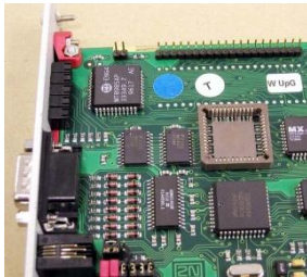
Position of the chip cap on the AUX board.
