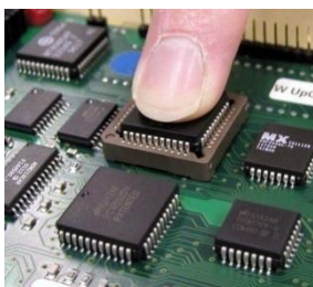
Carefully press the chip into the cap.
