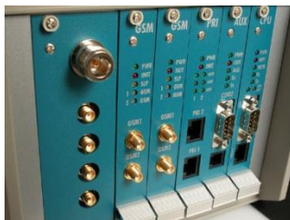
Internal Antenna Splitter for 2N® BlueTower
