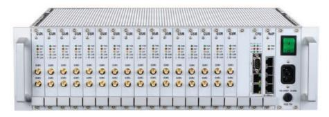
3. VoIP+ISDN: The gateway is configured to work both with the VoIP and ISDN PRI cards.
